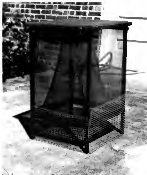
Fig. 12. Cone trap baited with 1-day-old fish heads to sample fly populations at compost plant.
