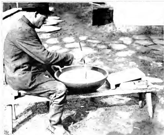
Fig. 239. After the steam and mud have been stripped from the Pans, the plaster is added and the mixture is stirred until the plaster begins to stiffen.
