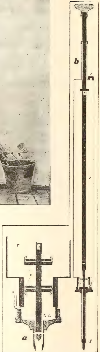
Fig. 48o, the McGowen injector in section, showing its working parts. Fig. 48r, illustrating method of using McGowen injector. Fig. 478, a knapsack sprayer.
