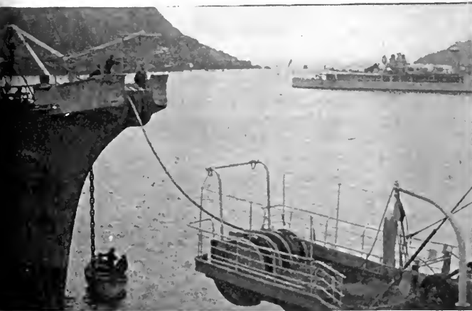
Here the cable is being transferred from the "Colonia" which brought the cable over from England to the "Cyrus Field" which handled the landing operations at Bay Roberts.
