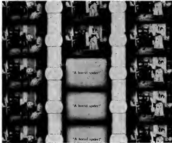
A specimen Home Kinetoscope film. The actual size is indicated above at left. Enlargement shows three parallel rows of pictures which were projected as the mechanism moved the film up and down its length.
