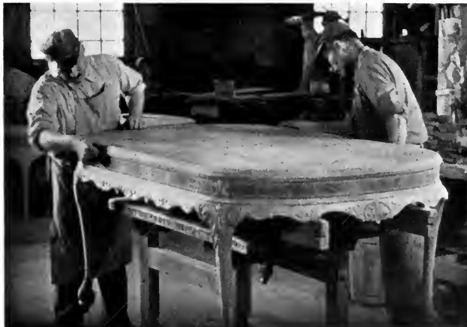
Workmen assembling a table top—from the Eastman classroom film, "Furniture Making."
