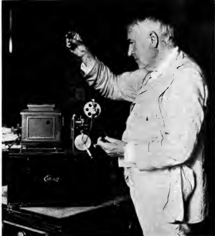
The Wizard of Menlo Park about 1913. He is giving final inspection to his then newly invented Home Kinetoscope made to serve a still undeveloped non-theatrical field.
