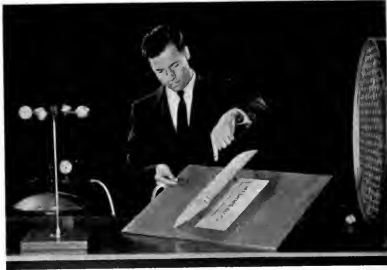
Demonstrating the effect of a swift current of air on top curved surface of plane's wing, in the Bray motion picture "Youth Takes to Wings."
