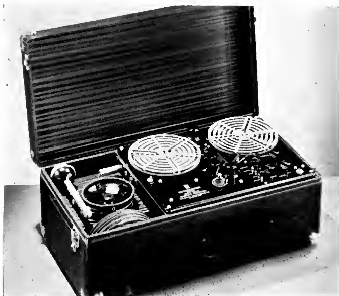
The new portable Brush "Soundmirror" recorder. This model (BK-403) has a low-speed drive for recording speech. A magnetic paper tape is used, which may be edited with a pair of scissors and some Scotch tape.
