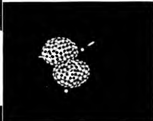
When a neutron hits a uranium nucleus, the nucleus splits in two, and other free neutrons are released. An entire chain of such reactions takes less than a millionth of a second.
