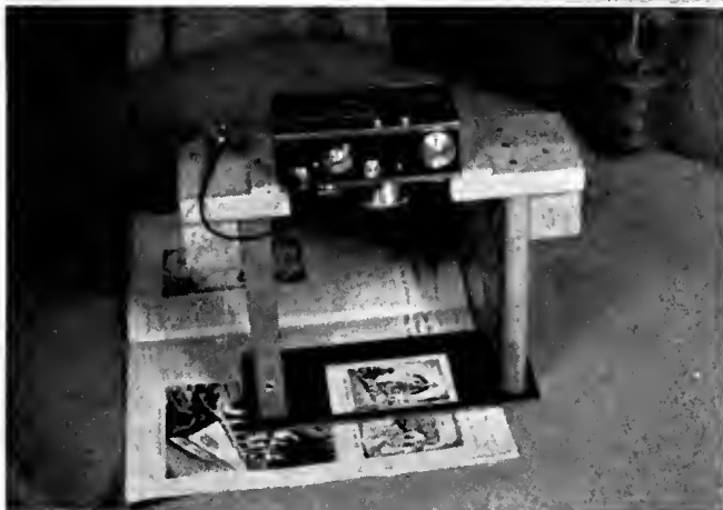
Home-made copy equipment for making 2 x 2 slides
