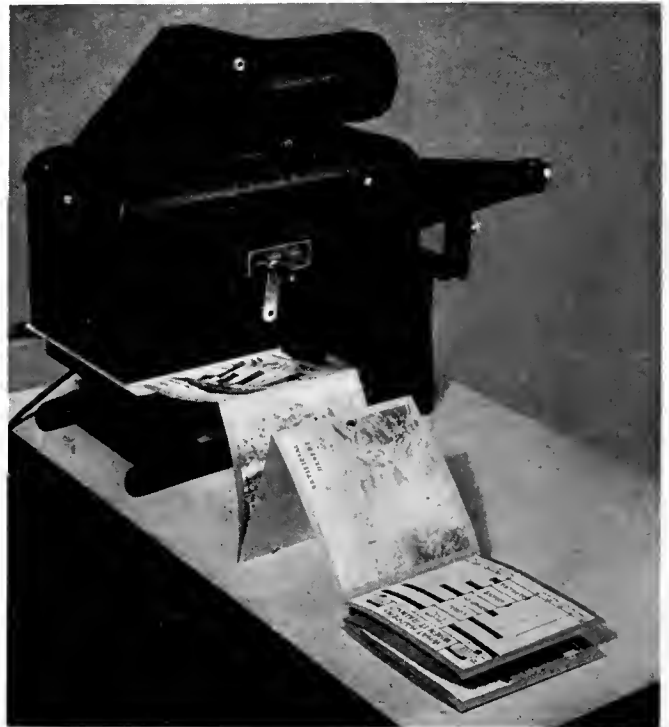
The user of this opaque projector has created a picture strip from magazine clippings. (Refer to Frank Walter's article, October, 1946, page 439). The projector is a Spencer Delineascope made by the American Optical Co. The Charles Beseler Co., New York City makes opaque projectors accommodating 8\frac{1}{2} "x11" pages.
