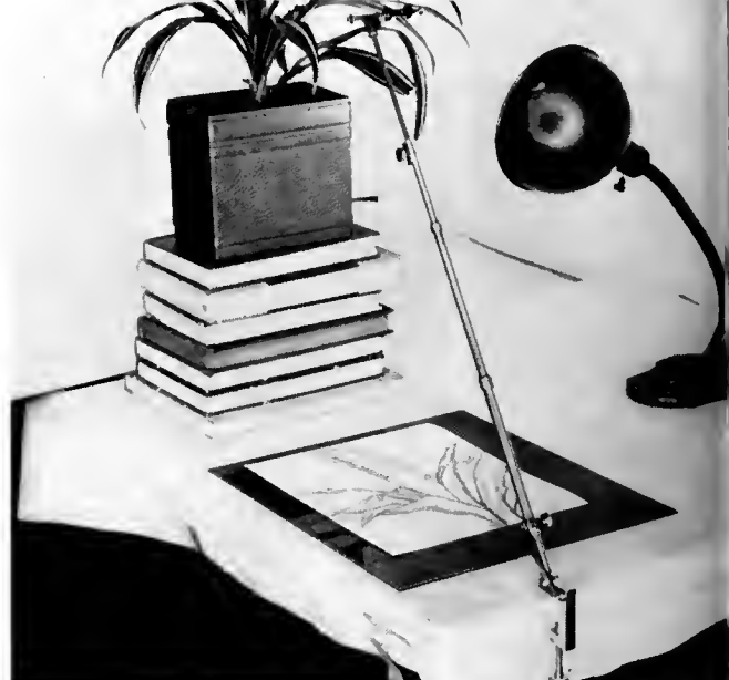
A commercial camera lucida. The 'home-made' arrangement costs far less, yet results compare very favorably with this unit. The prism can be tilted to a desired angle.
