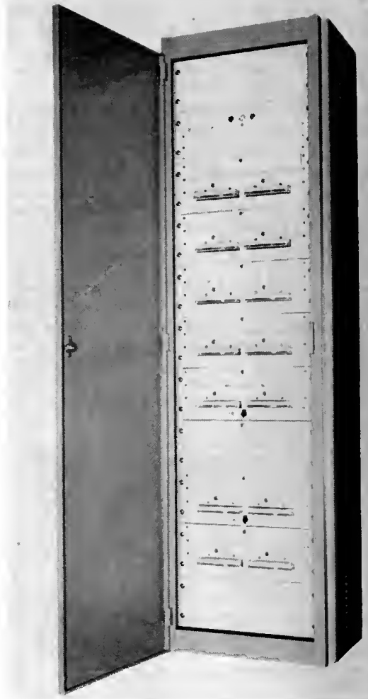
The remote control tape unit. This instrument, kept in an adjoining room, contains 30 dual track tape recorders.
