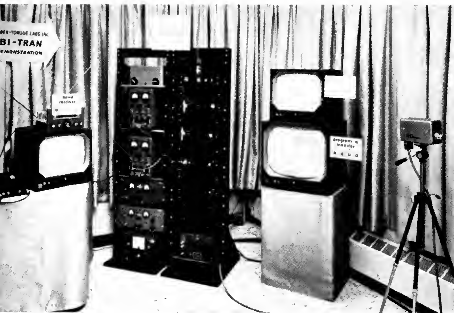
Figure 9. Experimental equipment to demonstrate the ability of a single TV channel to telecast two separate programs simultaneously. (Blonder-Tongue Laboratories)
