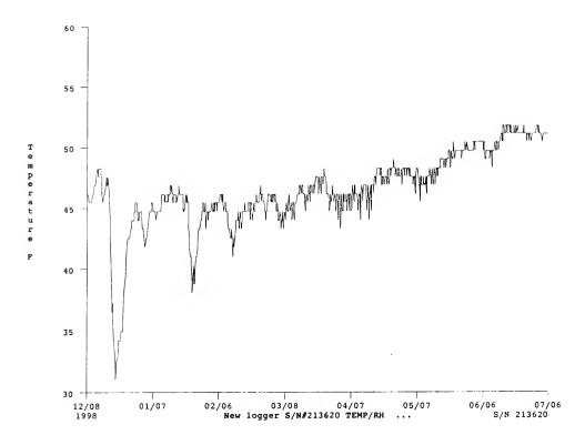
Figure 1. Mine temperature of the McDonald Mine East Adit (shallow location), Lake County, Montana, from December 1998-July 1999. Electronic data recorder was 39.7 m from the mine portal.
