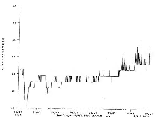
Figure 5. Mine temperature of the McDonald Mine West Adit, Lake County, Montana, from December 1998-July 1999. Electronic data recorder was 12.7 m from the mine portal.
