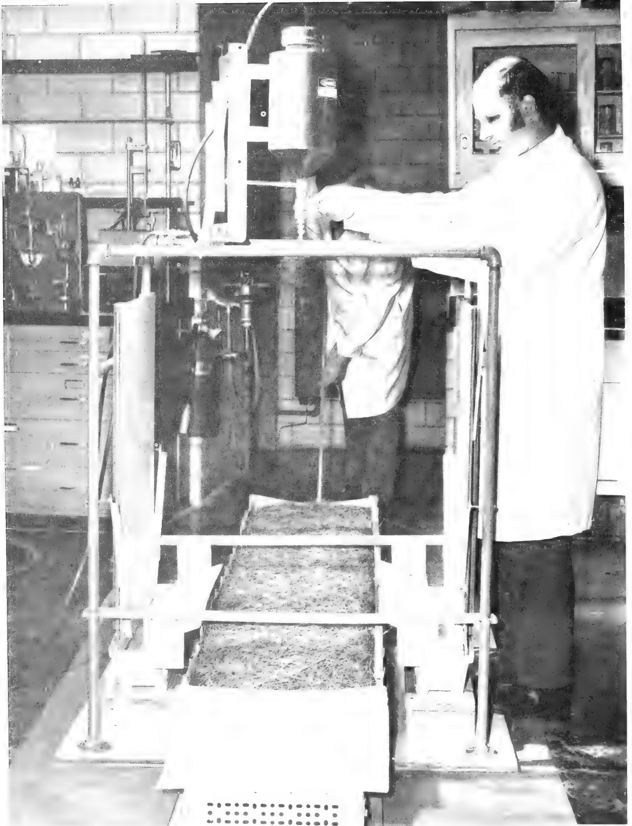
Figure 2.--Spray system in operation.
