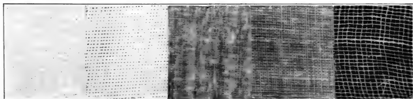
FIG. 2.—REPRODUCTIONS FROM PHOTOGRAPHIC PRINTS, SHOWING THE TEXTURE OF THE CLOTHS USED ON SECTIONS 1 TO 5 AND INDICATING THE RELATIVE LIGHT PENETRATION.
