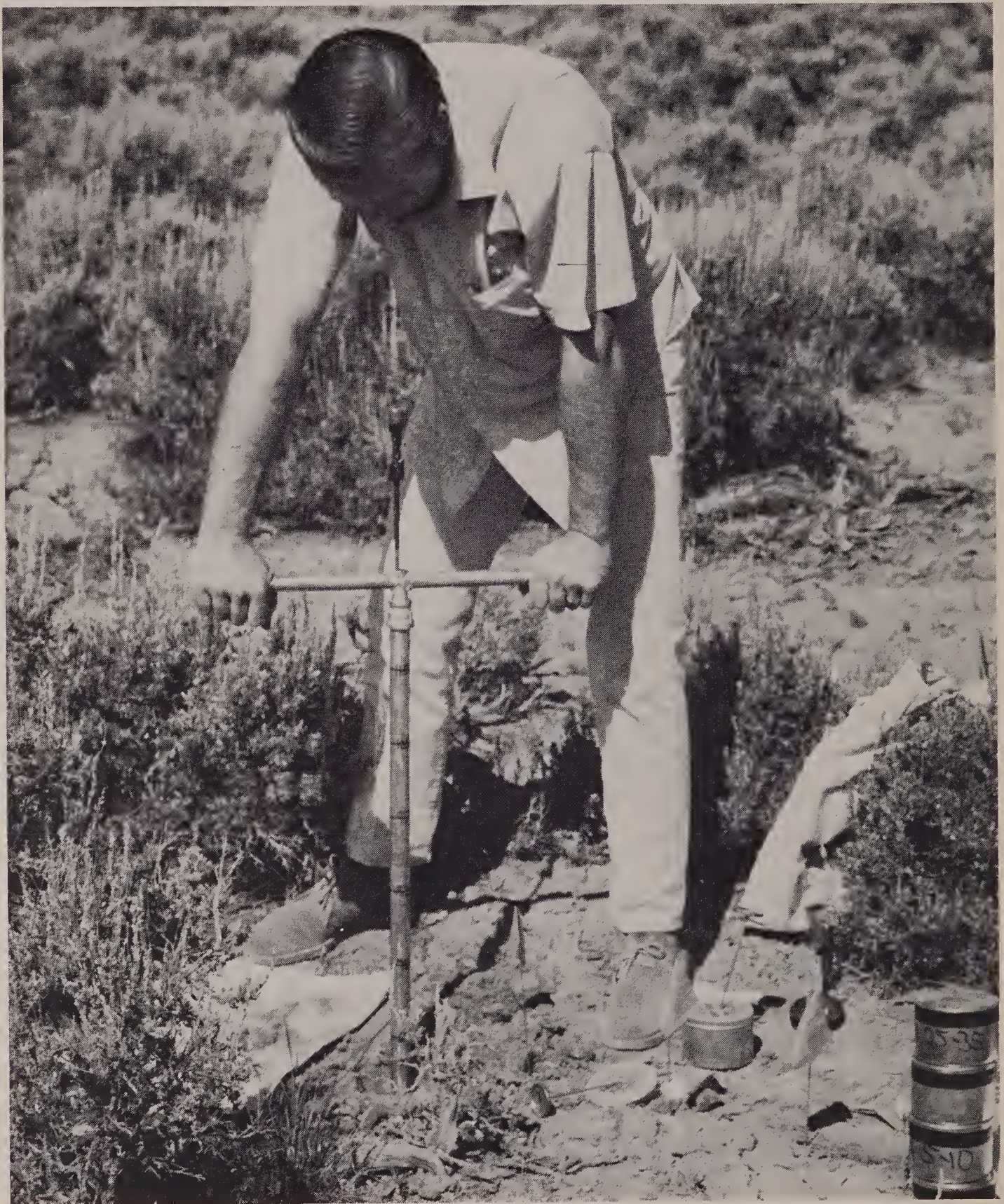
FIGURE 4.—Acquisition of soil samples for determination of soil moisture.
