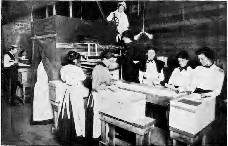
An Extraordinary Egg-Candling Machine, whereby over Twenty-six Thousand Eggs an Hour can be Examined.
