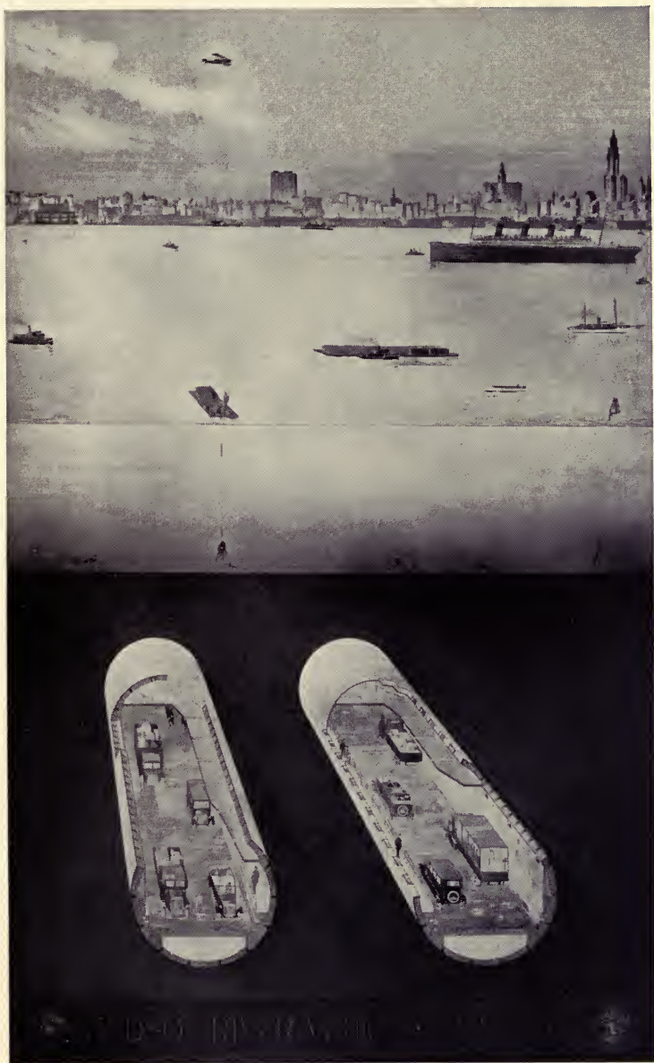
SECTIONAL VIEW OF HOLLAND TUNNEL Under the Hudson River, looking toward New York City
