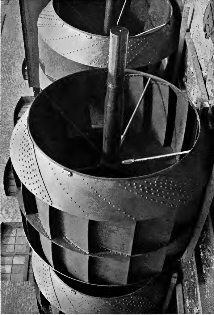
STURTEVANT SILENTVANE FAN WHEELS FOR THE HOLLAND TUNNEL
