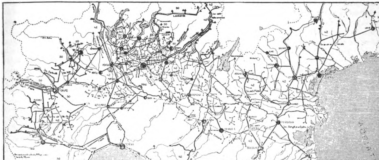
MAP OF NORTHERN ITALY SHOWING CENTRAL STATIONS AND ELECTRIC TRUNK LINES
