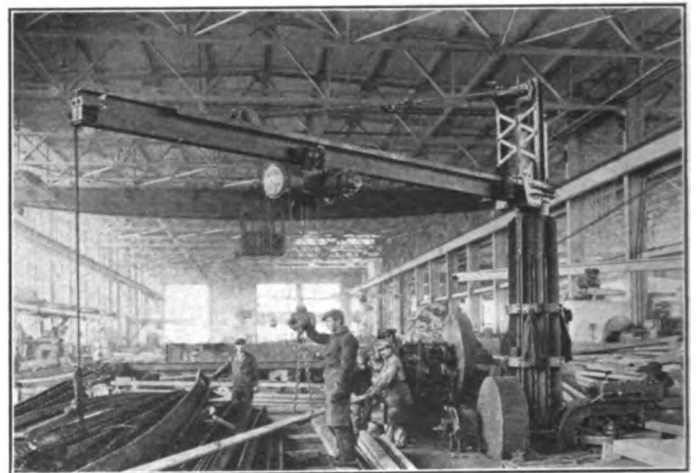
Self-supporting bracket crane, 3 tons, serving a heavy punch used for punching deck beams and ship frames. Fore River Shipbuilding Corp., Quincy, Mass.
