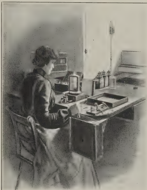
Flashing the Lamps. A Screen Hides the Lamp from the Operator's Direct Vision.
