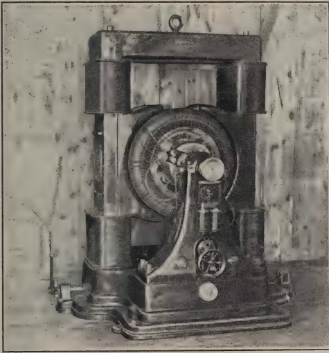
Arc Dynamo Used to Operate the Nitrifier.
