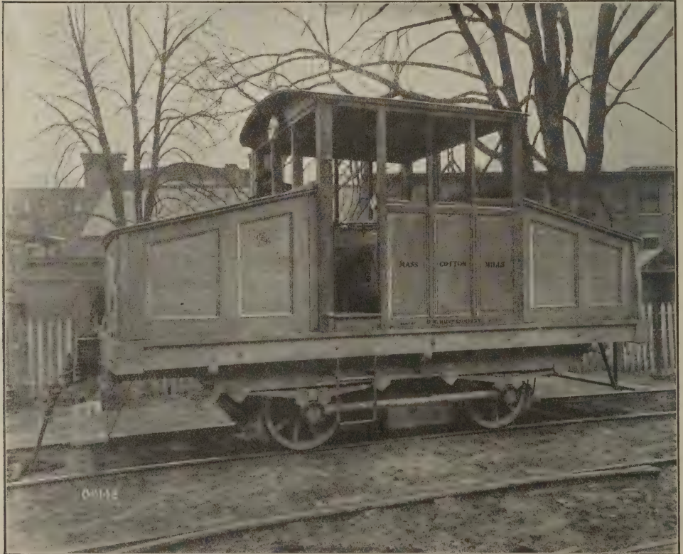
FIG. 4. 20-TON Electric Storage Battery Locomotive.
