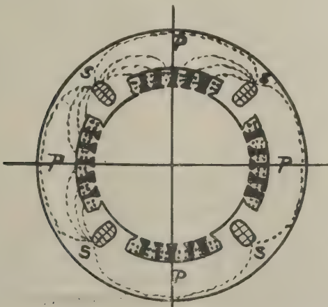
FIG. 5. AUXILIARY STARTING COILS FOR HEYLAND SINGLE-PHASE MOTOR.
