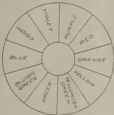
FIG. 1. SCHEME FOR COLOR MIXTURES OF LIGHT.
