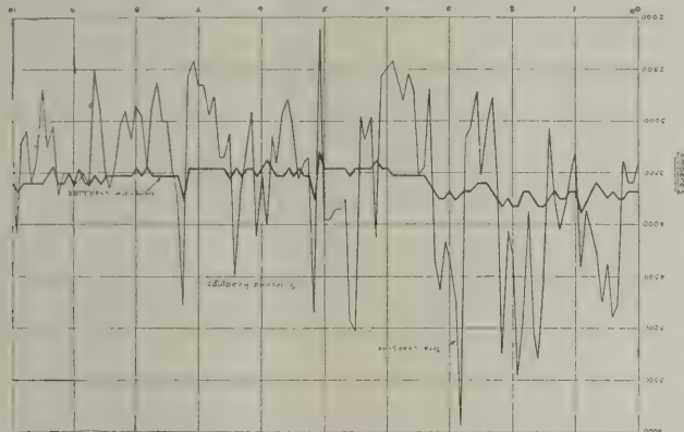
FIG. 4. LOAD CURVE OF SAME PLANT AFTER AN ADDITION INCREASING LOAD BY 500 K. W. AND AFTER THE INSTALLATION OF A STORAGE BATTERY.
