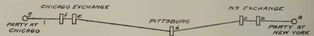
FIG. 1. SCHEME OF CONNECTIONS FOR A CALL BETWEEN NEW YORK CITY AND CHICAGO.
