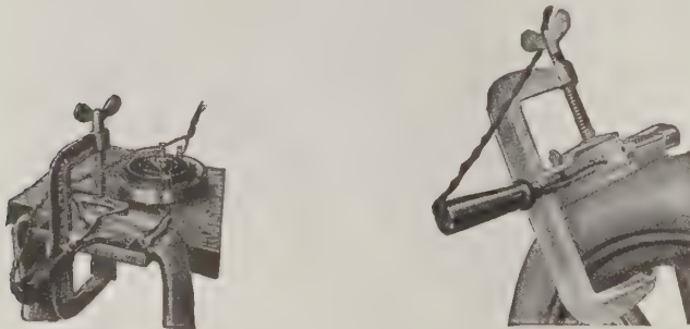
FIG. 4. ELECTRIC VULCANIZING OUTFIT.
