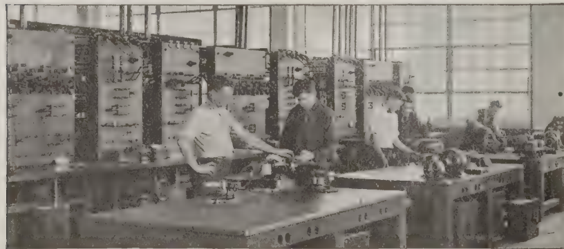
FIG. 7. TESTING SMALL MOTORS IN PLANT OF WESTINGHOUSE ELECTRIC & MFG. COMPANY.
