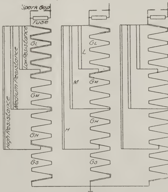
FIG. 1. CONNECTIONS FOR Y SYSTEM WITH GROUNDED NEUTRAL.
