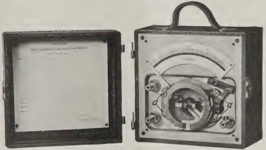
NEW WESTINGHOUSE PORTABLE AC AND DC METER, WITH COVER PLATE REMOVED.
