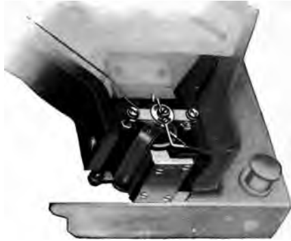
FIG. 22. — Movement of Weston Standard Voltmeter.
