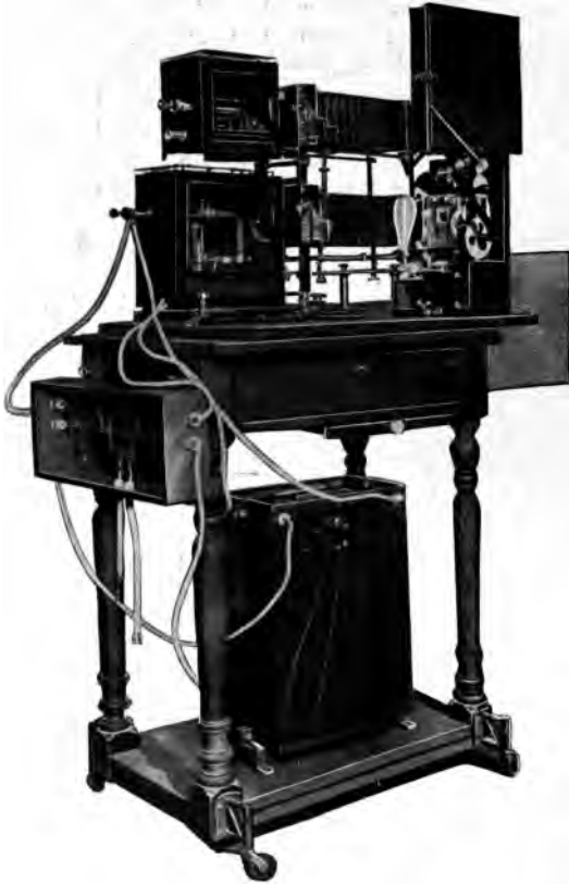
FIG. 420. — Combination Beseler Double Lantern and Moving Picture Apparatus. one thumbscrew is released, another thumbscrew is unscrewed, and its screw is removed. It is then possible to move the upper carbon holder forward so that its gear meshes with the inner gear on the lower carbon holder. This gear has the same number of teeth as the upper gear, and consequently both carbons may be fed together at the same rate.
