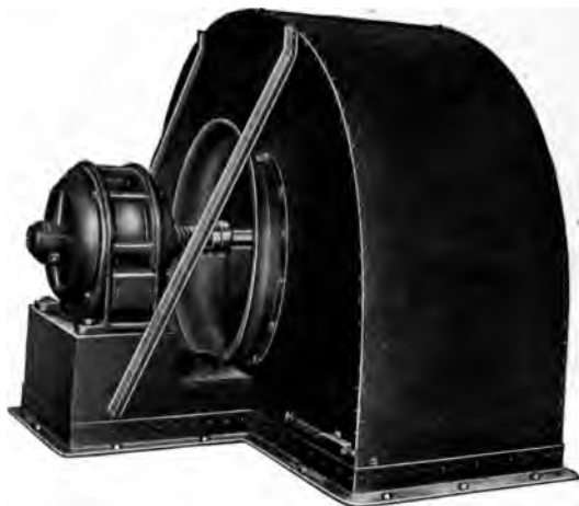
FIG. 397. — Induction Motor operating a Blower.
