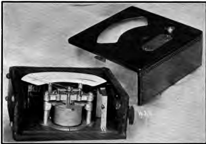
FIG. 318. Interior of Weston Alternating Current Voltmeter.
