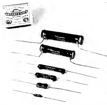
Plate 20.4 General purpose wirewound resistors, conservatively rated at 15, 10, 6, 4\frac{1}{2} , 3 and 1\frac{1}{2} W. Considerably higher dissipations than these are possible, e.g. 6 W in the 3 W size and 30 W in the 10 W size
