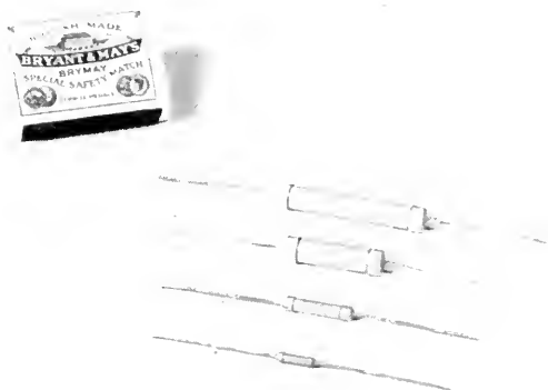
Plate 20.3 Pyrolytic resistors, rated at 2, 1, \frac{1}{2} and \frac{1}{4} W
