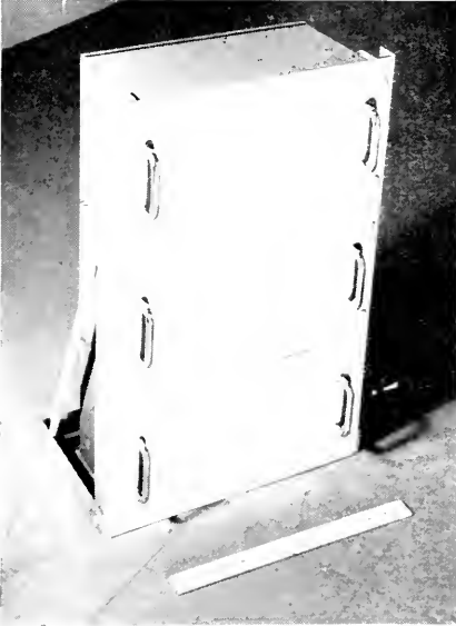
Plate 26.3 14 in. chassis and panel construction. Three blank units, each comprising chassis, panel, and dust cover are shown mounted on a rack
