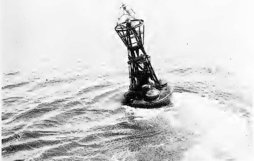
FIGURE 2-10.—A typical marker radiobeacon on a lighted buoy.
