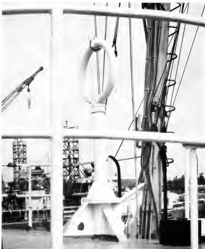
FIGURE 2-11—Weatherproof housing of a modern radio direction finder loop antenna mounted above deck.
