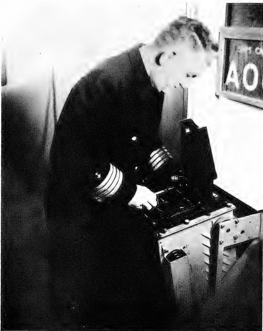
FIGURE 1-7.—Ship's captain obtaining positional data from a compact, lightweight type Loran receiver-indicator.
