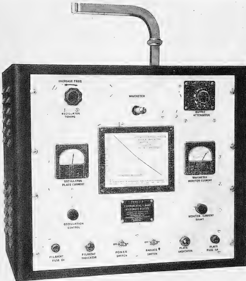
FIGURE 3-5.—X-band Ramark transmitter.
