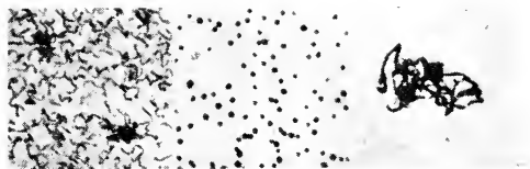
FIG. 33. Photographic grains. Magnification \times 125,000 (By courtesy of the Eastman Kodak Research Lab.)
