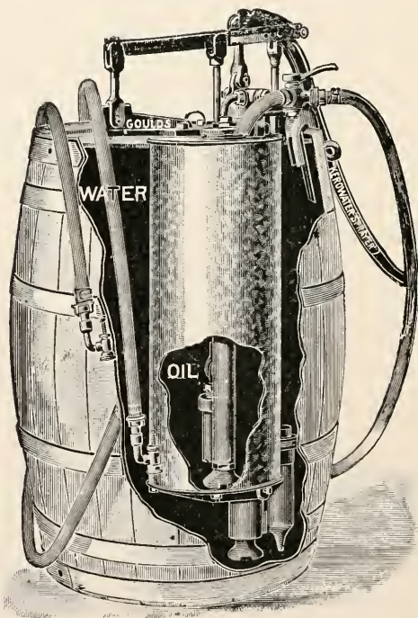
FIG. 232. "Kerowater" spray-pump. Designed for mechanically mixing and spraying kerosene and water. The oil and water are mixed and discharged in a milk-like emulsion.
