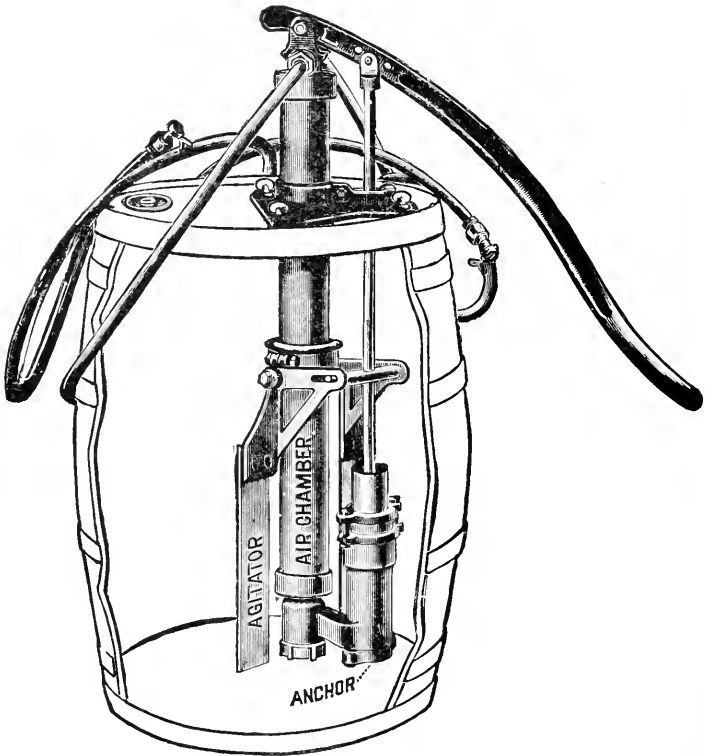
FIG. 231. The "Pomona" spray-pump, mounted on end of barrel. Used to spray with arsenical mixtures.
