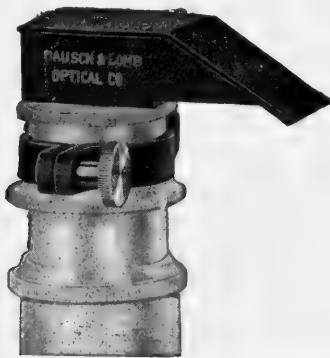
FIG. 73.—Camera Lucida, Fixed Mirror Type. (Bausch & Lomb.)
