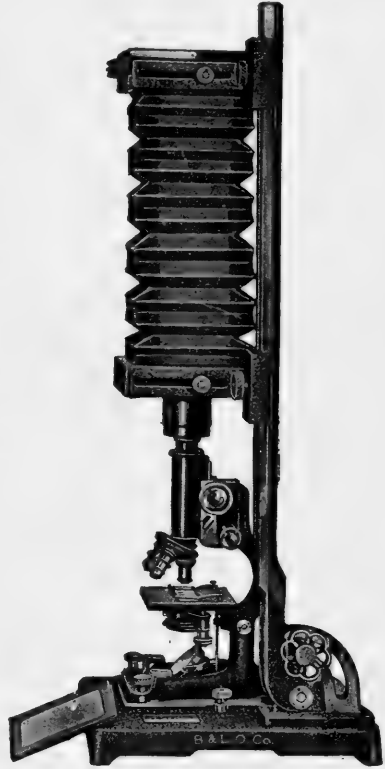
FIG. 26.—Microphotographic Apparatus. (Bausch & Lomb.)
