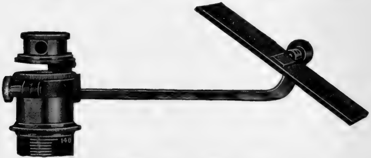
FIG. 72.—Camera Lucida, Adjustable Mirror Type. (Bausch & Lomb.)
