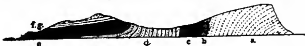
FIG. 1.—Section of the Isle of Wight—a Monocline Curve. a , Chalk; b , Woolwich and Reading beds; c , London clay; d , Bagshot series; e , Headon series; f , g , Osborne and Bembridge series.
