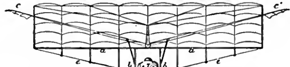
FIG. 43.—A similar system, planned by Wenham. a, a, Main spar 16 ft. long; b, b, Panels, with base board for aeronaut attached to main spar. e, e, Thin tie-band of steel with struts starting from main spar. This forms a strong light framework for the aeroplanes, consisting of six webs of thin holland 15 in. broad. The aeroplanes are kept in parallel plane by vertical divisions of holland 2 ft. wide. c, c', Wing propellers driven by the feet.
