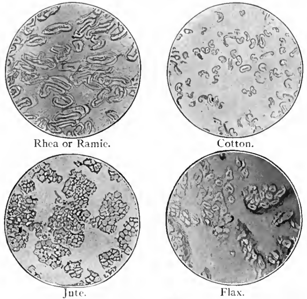
FIG. 10.—COTTON. FLAX. RAMIE. JUTE. Ultimate fibres—transverse section, \times 110 . Note similarity of ramie to cotton and jute to flax. Jute "fibre," a filament formed of compact agglomerate of ultimate fibres, contrasts with flax, in which ultimate fibres only slightly adherent—hence its divisibility and "drawing" quality under hackling and spinning treatments.
