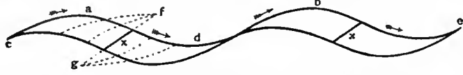
FIG. 13.—Wave track made by the wing in progressive flight. a, b , Crests of the wave; c, d, e , up strokes; x, x , down strokes; f , point corresponding to the anterior margin of the wing, and forming a centre for the downward rotation of the wing ( a, g ); g , point corresponding to the posterior margin of the wing, and forming a centre for the upward rotation of the wing ( d, f ).
