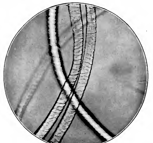
FIG. 4.—WOOL FIBRES. Australian merino viewed in length, \times 235 . Surface imbrications—the structural cause of true felting properties.
