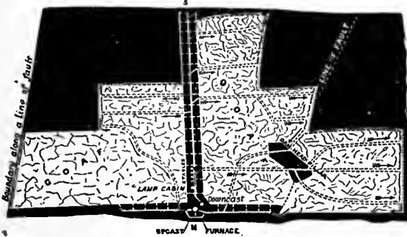
FIG. 7.—Long-wall method of working Coal in Derbyshire.
