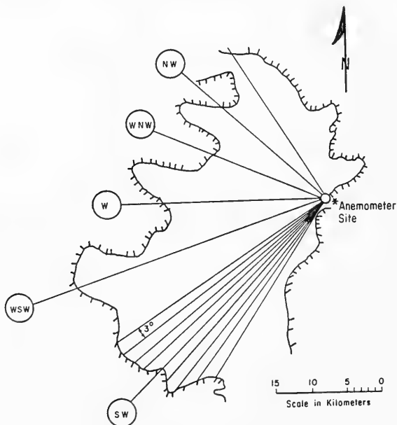
Figure 5. The fetch length for this irregularly shaped water body in the wind direction is determined by drawing nine radials at 3° increments centered on the wind direction and arithmetically averaging the radial lengths as illustrated. The average fetch in this example is approximately 22.2 miles (36 kilometers).
