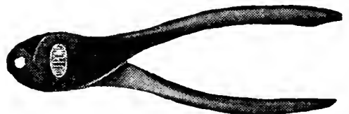
FIG. 159. Cap crimper and fuse cutter, one handle of which will serve to make the cap opening in the stick of dynamite
