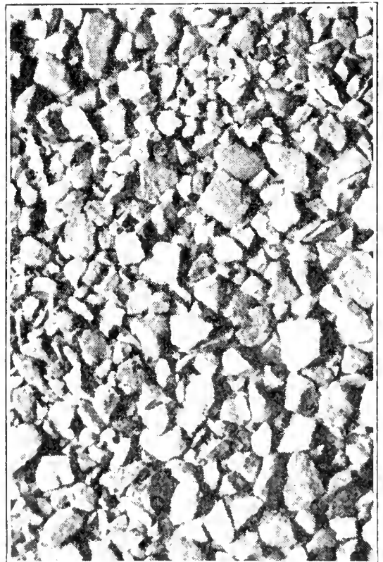
FIG. 131. Limestone screenings that may be used in concrete work in place of sand
