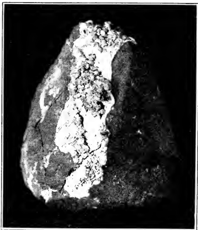
FIG. 133. Concretion that is frequently found in gravel too weak for use in concrete
