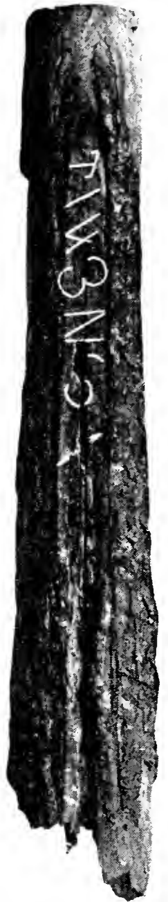
FIG. 105. Markings on one of the bearing trees for the section corner shown in Fig. 104
