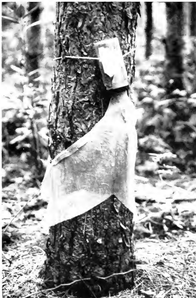
Figure 1. Aluminum screen trap with glass jar used to collect I. Novaboracensis adults.
