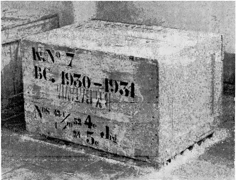
Fig. 6. Book-chest made of inferior wood which has become severely infested by Heterobostrychus aequalis in a cellar in Bogor, Java. Mark the cones of frass piling up along the bottom.
