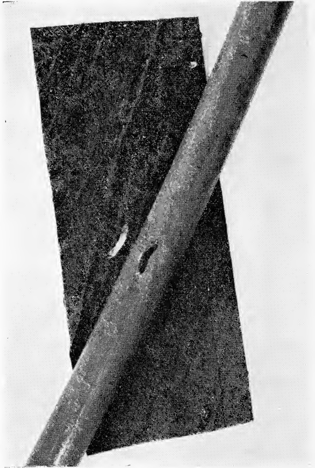
Photo K. Inst. v. d. Tropen Perforation by Coptotermes of the leaden sheath and the enveloping tarred paper in the core of a telephone cable (nat. size)
