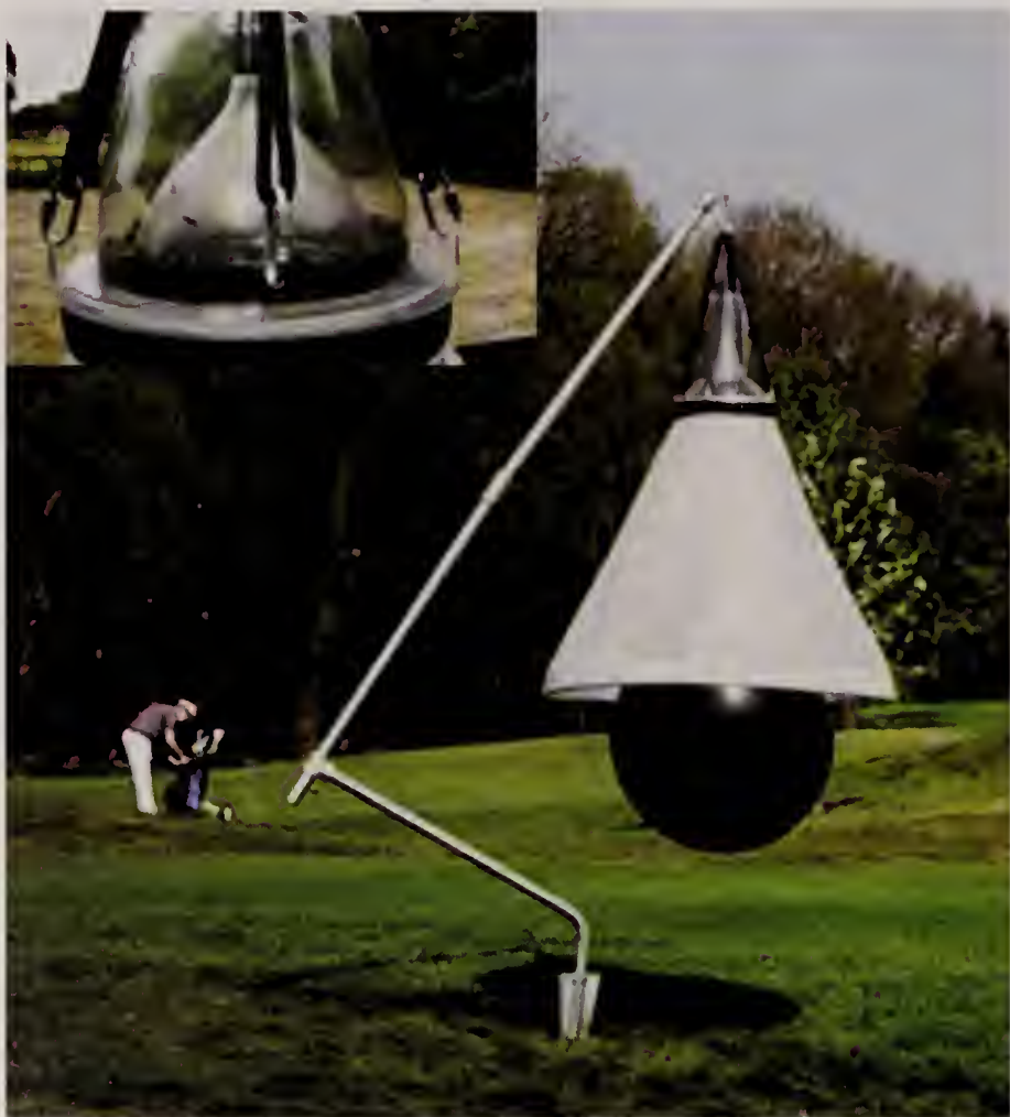
15. Ball and hood (LOER-2007) trap for collecting horse flies. Left the collector with flies killed by heat. From: www.dazenval.nl
