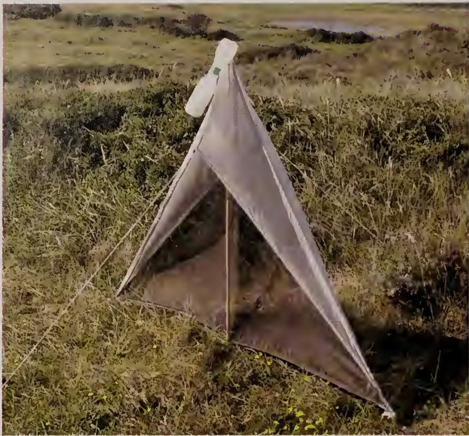
13. Bilateral Malaise trap with triangular opening and a central collector. Photo: J. de Rond
