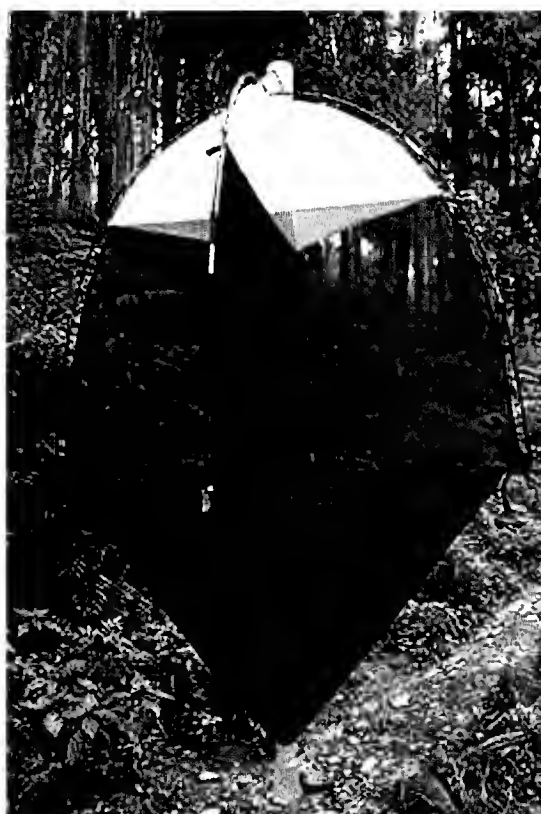
11. SLAM (Sea Land & Air Malaise) trap version with a top and a bottom collector for suspending in trees (from: http://bugdorm.megaview.com.tw ).
