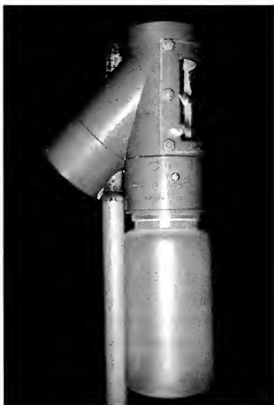
9. Small grey 50 mm PVC collector for Malaise traps with 0.2 l bottle. Photo: C. van Achterberg
