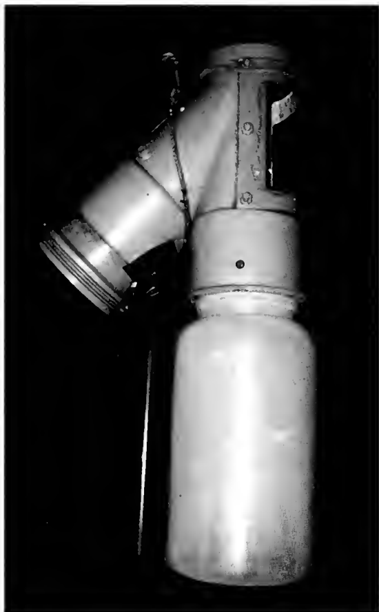
8. Large grey 75 mm PVC collector for Malaise traps with 1 l bottle. Photo: C. van Achterberg
