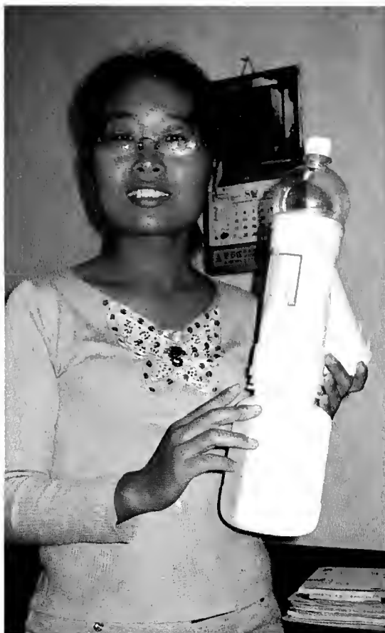
10. Large white 75 mm UPVC (Unplasticised PolyVinylChloride or rigid PVC) collector for Malaise traps (Hangzhou type) with 1 l bottle. Photo: C. van Achterberg
