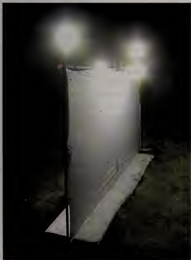
2. Four lamps of 500 W each light a vertical white polyester sheet of 1.9 × 3.5 m. Another white sheet is positioned on the ground. Photo: Paul van Wielink
