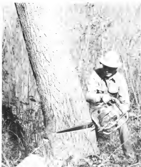
FIGURE 1.—Felling with one-man powersaw.
