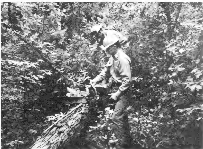
FIGURE 2.—Limbing tree and marking bole for bucking with a two-man crew.
