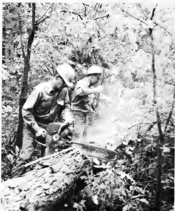
FIGURE 3. — Bucking bole into logs with two- man crew: One man saws while the other clears away brush and limbs.
