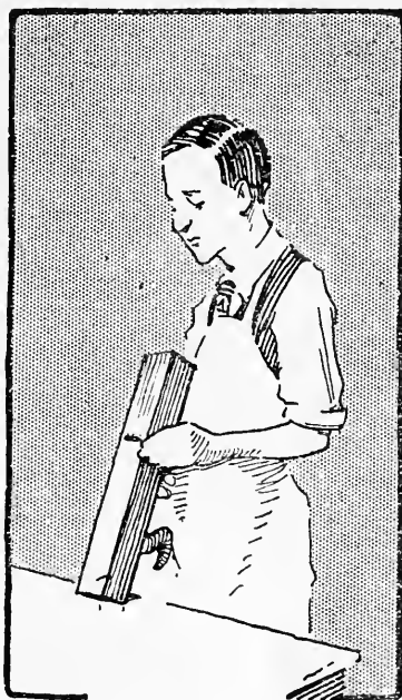
Fig. 26.—Sighting along Sole of Plane for Projection of Cutter
