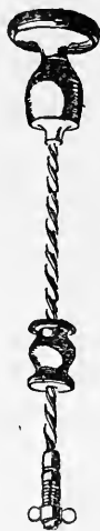
Fig. 5.—Archimedean Drill with Chuck or Holder to take Drills or Boring Bits
