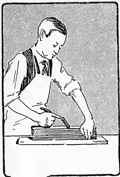
Fig. 27.—How to hold the Jack Plane
