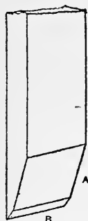
Fig. 20.—End of Chisel, showing Grinding Angle (A) and Sharpening or Setting Angle (B)
