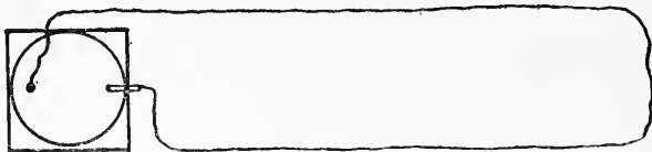
Fig. 2.—Cell and Simplest Circuit
