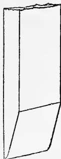
Fig. 20A.—Showing how Edge of Chisel is spoiled by Bad Setting; note the Rounded Angle
