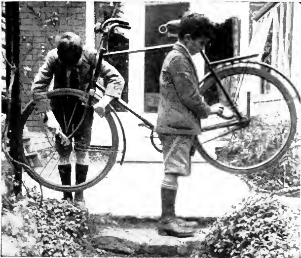
Bicycle Suspended by Rope for ease in Oiling and Adjustment
