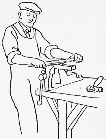
Fig 8.—Position for Draw-filing
