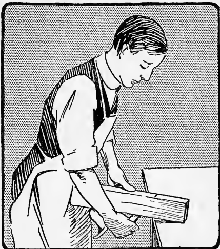
Fig. 14.—Striking Plane on Bench to loosen the Wedge
