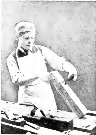
Testing Planed Wood Across the Grain
