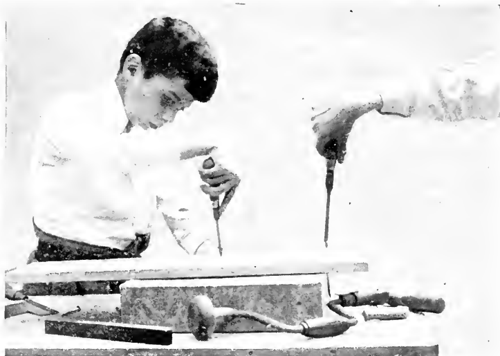
Narrow Screwdriver Injures the Screw-head
