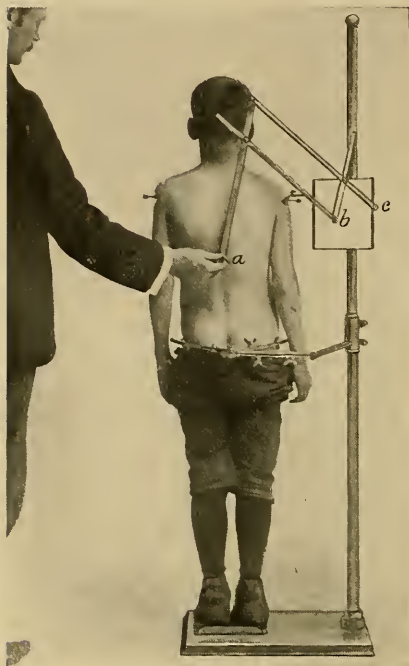
Fig. 346.—Making a tracing of the lateral deviation by the author's scoliosimeter: a , Pointer which follows the line of the spinous processes and tips of the scapula; b , pencil recording the tracing on paper to the scale of 1 to 4; c , fixed point of the pantograph.
