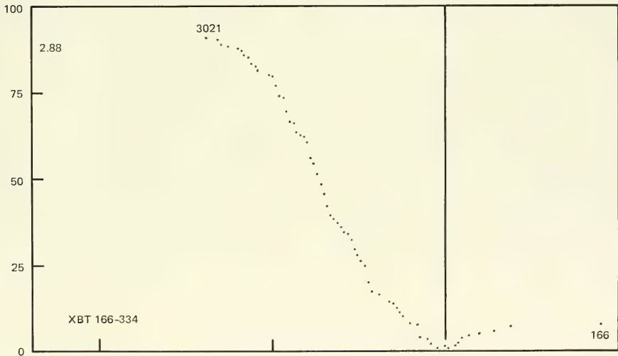
Figure 16. Ogives of positive and negative differences between Gulf of Alaska XBT surface temperatures and towed thermistor temperatures.
