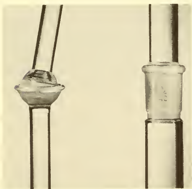
Fig. 5-1. Left, standard ball joint; right, standard taper joint. (Courtesy Corning Glass Works.)
