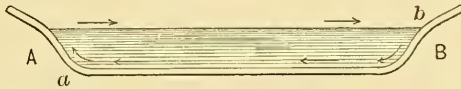
FIG. 51. — Vertical section through a dish showing distribution in water of passively suspended bodies, as a result of difference of temperature at the two sides of the vessel. A , warmer side; B , cooler side. Arrows show the direction of movement of currents in the water. The objects lighter than water are grouped at b ; those heavier than water, at a .
