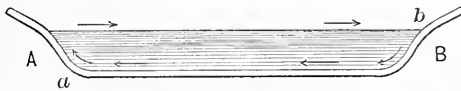
FIG. 51. — Vertical section through a dish showing distribution in water of passively suspended bodies, as a result of difference of temperature at the two sides of the vessel. A , warmer side; B , cooler side. Arrows show the direction of movement of currents in the water. The objects lighter than water are grouped at b ; those heavier than water, at a .
