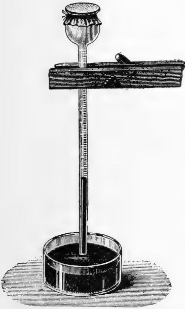
Apparatus to demonstrate lifting power of evaporation. (After Oels.)
