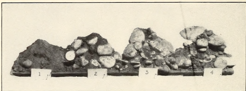
FIG. 2.—SAMPLES OF FIRST, SECOND, THIRD, AND FOURTH FOOT OF VERY GRAVELLY SOIL.
