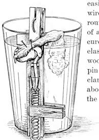
70. Apparatus for determining the force of growth of a root by means of a spring.
