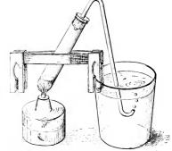
105. Apparatus for the decomposition of starch; the gases pass into a tumbler of lime-water.
