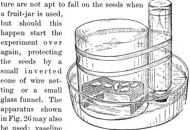
27. Method of maintaining a saturated atmosphere and a constant water-level.
