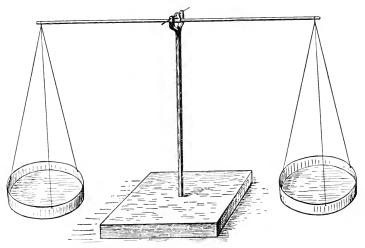
A home-made balance constructed of umbrella wire; it can be made sensitive to a tenth of a gram.
