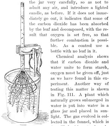
111. Arrangement for collecting the gas given off by a water-plant in sunlight.
