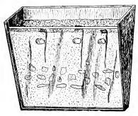
80. Apparatus for observing the behavior of roots as they encounter obstacles.
