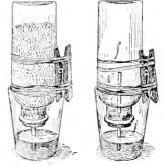
31. Method of measuring the amount of carbon dioxide produced by germinating seeds, the tumblers contain lye (control at the right).
