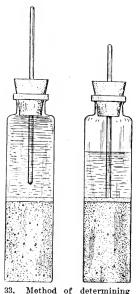
Method of determining whether air exists in the soil.
