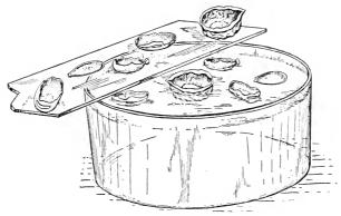
Seed-covers floating on water, each containing a few sugar crystals, which, by dissolving, indicate the rapidity of osmosis; controls on the glass strip.
