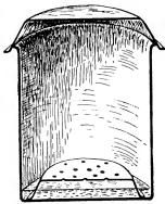
206. Steam sterilizer, consisting of a pail, a pan for cover and a smaller pan pierced with holes as a support (all should be of tin or agateware). (Sectional
