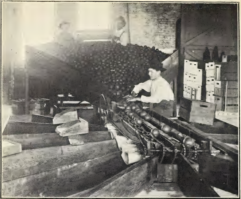
FIG. 1.—TYPE OF ORANGE SIZER, HOPPER, AND BINS USED IN THE OLD PACKING HOUSES IN FLORIDA.
