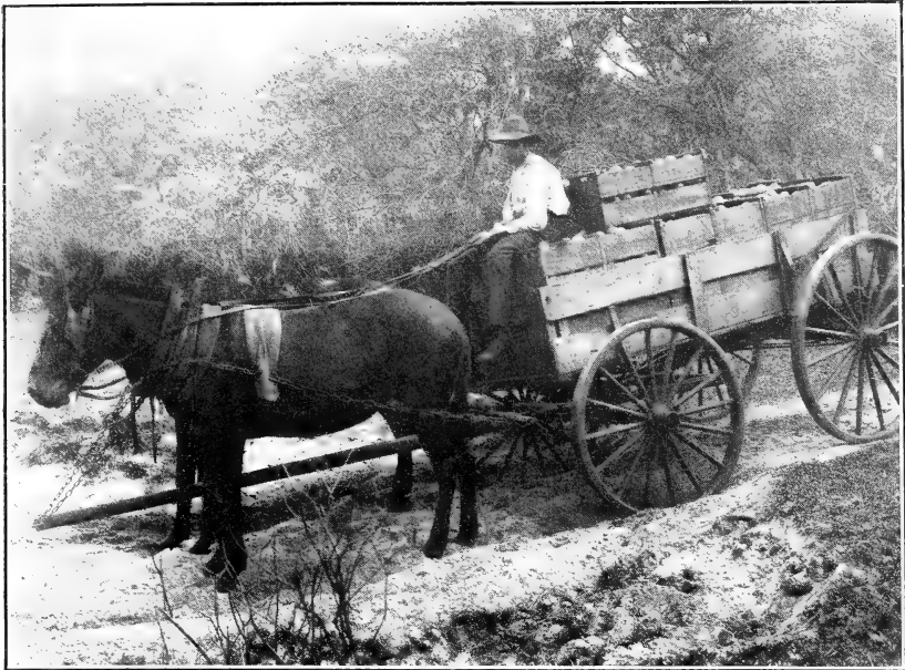
FIG. 1.—HAULING ORANGES OVER ROUGH ROADS ON WAGONS WITHOUT SPRINGS. The jolting and jarring and the driver seated directly upon the fruit result in serious injury.
