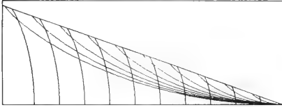
Fig. 6 — The Classical Kelvin Ship Wave Pattern
