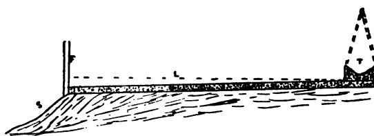
FIG. 390. CEMENT FEEDING FLOOR FOR HOGHOUSE.
