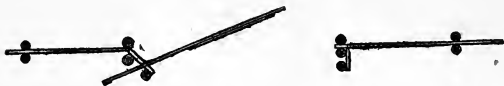
Figure 65.—Plan Showing Fence, Fence Posts and Field Gate. The Posts Should Be So Placed as to Permit the Gate to Open At Right Angles to the Fence
